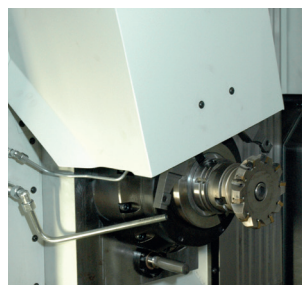
Automatic tool changer with double gripper
