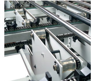
Step chain belt with a longitudinal roller conveyor and left-aligned workpiece limit stop for processing the first side, and a right-aligned workpiece limit stop for processing the second side
