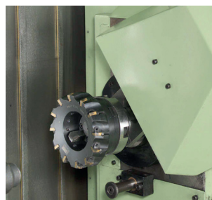
Automatic tool changer with double gripper
