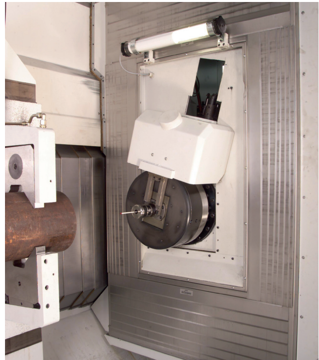
CNC controlled facing head with integrated electrical balancing system
