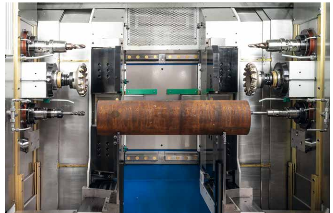
Processing on both sides possible! As standard, up to 3 tool spindles are implemented per side.
